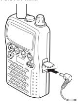
5 Insert the AC adapter power plug into an AC outlet (100 V-240 V).
